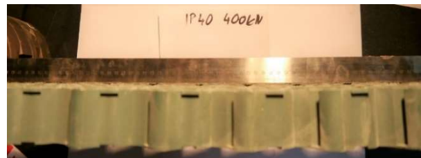
Photo.6. IP 40 after the test at 400kN
