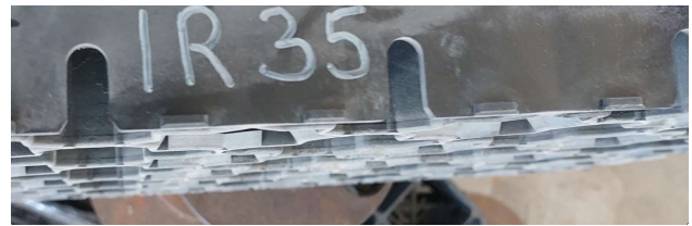
Photo.4. IR 35 after test at 80kN
