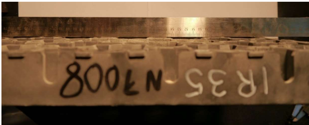
Photo.7. IR 35 after test at 800kN
