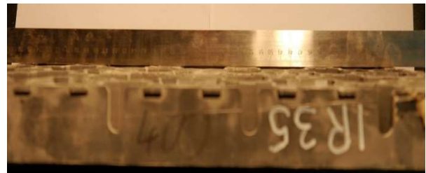
Photo.6. IR 35 after test at 400kN
